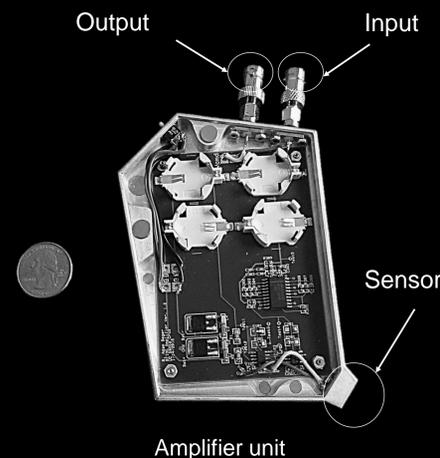
Since the corded connection of the amplifier unit hindered the mobility nature of the biosensor unit, the transmission medium was changed to a wireless device.
