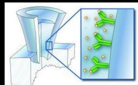
STING technology relies on a simple electrochemical readout that transduces, in a label-free manner, binding events at the tip of a functionalized nanopipette. Antibodies, DNA and aptamers have been used as recognition elements demonstrating the versatility of this platform for biorecognition. [1]
